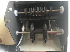
b) Loose the screw on the bottom of the power board ;take off the small motor chain., Take off the screws as picture by"+" shape screwdriver, take out the turning wheel. Take off the small motor,Pull out the connecting wire from the hole after take off the small motor.
