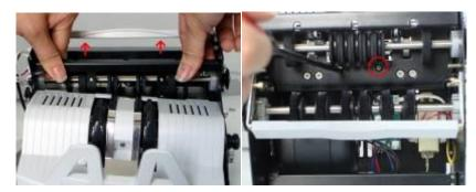
c) take out the counting sensor and magnetic head, pull the wire from the hole ,then take off the screw on the send sensor. Fix all up after replace.
