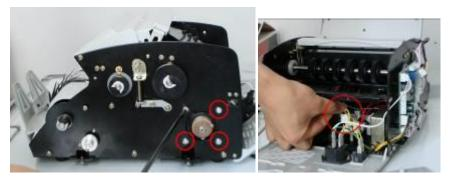
**b**) Take off the main motor from back of the machine, take off the screw. Replace the main motor , then fix all up. Connect to the power ,test if it work well.
